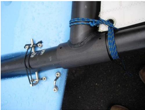
If you are having trouble positioning the inner bar – put the trampolines roughly in position and align the bars with that. Make sure you leave enough of a gap so that you can tension the trampoline properly
