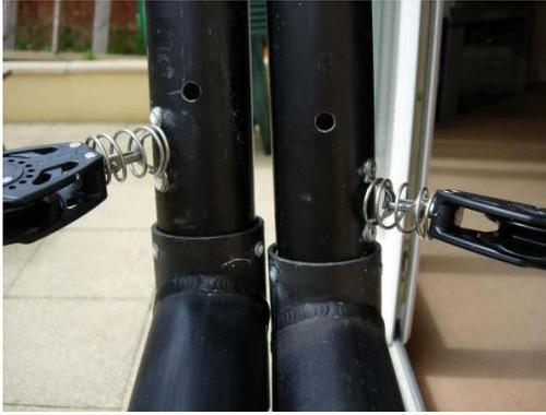
Assemble the innerbar . . . your wings may not be entirely symmetrical – but make sure that the inner wing bar is going to be in the same position with respect to the gunwhale on each side.
