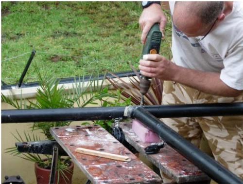
Drill out rivets on inner bar. Leave the outer bar attached (unless you are upgrading this as well). Remove all the other fittings on the front strut that are inboard of where the joints will go (toestraps, spinnaker blocks, etc.)
