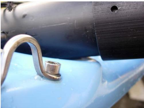
Slide the inner wing bar up the struts until it is roughly in the correct place.
