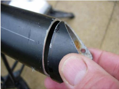
You need to shorten the existing inner bar by cutting off the shaped piece at each end.
